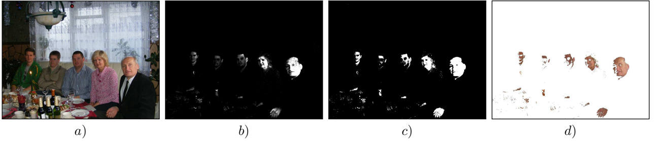
Figure 3.27: Output from naïve Bayesian skin classifier trained using Jones and Rehg’s (2002) dataset. Image a ) shows the original input, image b ) shows \frac{\Pr(\text{skin}|\text{rgb})}{\Pr(\neg\text{skin}|\text{rgb})} , this ratio is thresholded in image c ) obtaining a binary mask, and the original image filtered using this binary mask is shown in d ).
