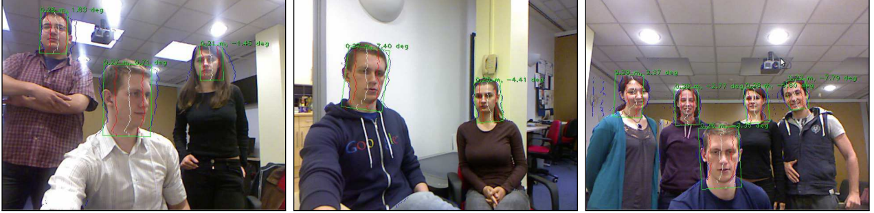
Figure 3.49: Multiple head detection examples using the proposed extension of Garstka and Peters' method.
