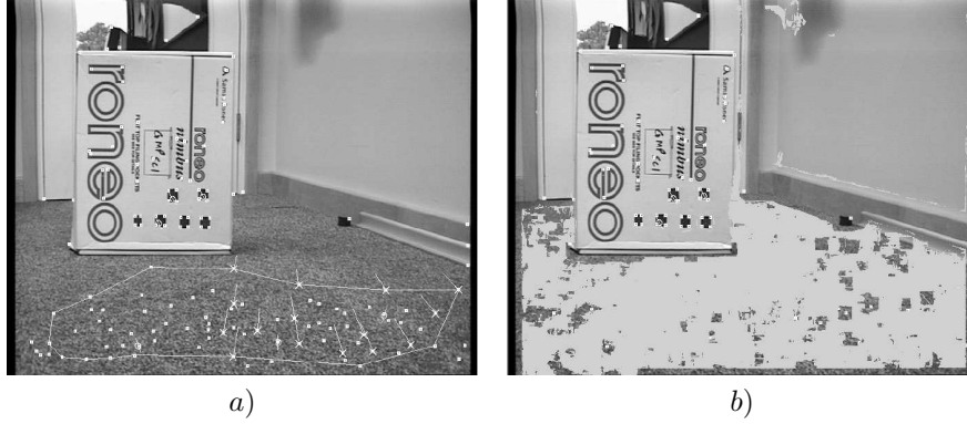
Figure 3.41: Ground plane segmentation in Pears and Bojian's (2001) method, based on calculation of the homography that relates ground planes in temporally separated frames. Image a ) shows the extracted corner points on the ground plane grouped into a patch, image b ) shows the extracted ground plane region, based on its colour similarity to the colour of the patch in image a ). Adapted from Pears and Bojian (2001).
