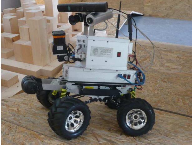
Hector, an unmanned ground vehicle for autonomous victim search and environment mapping. Taken from Graber et al. (2013).
