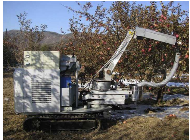
An autonomous apple harvesting robot. Taken from De-An et al. (2011).
