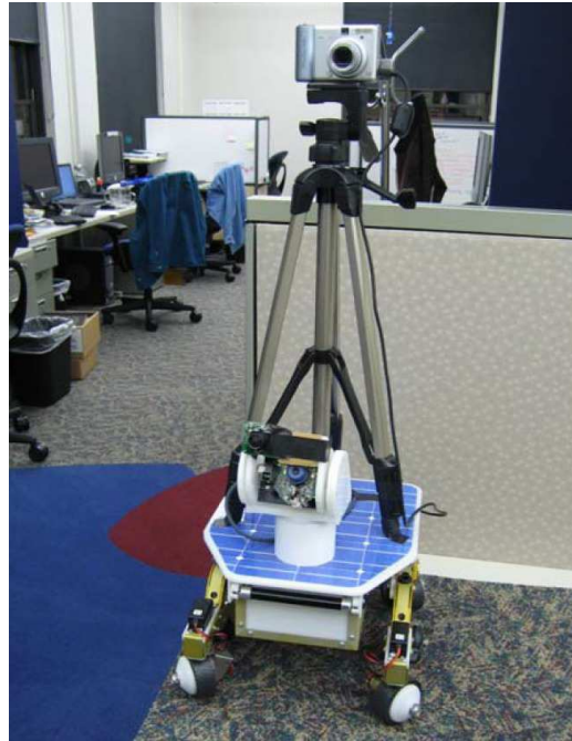
Figure 2.2: Table-top robot capable of group picture framing using optical flow. Taken from Campbell and Pillai (2005).
