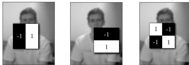
Figure 3.8: Two-dimensional Haar wavelets with square support, as described by Papageorgiou and Poggio (2000). From left to right: vertical, horizontal and diagonal 2D Haar wavelets.
